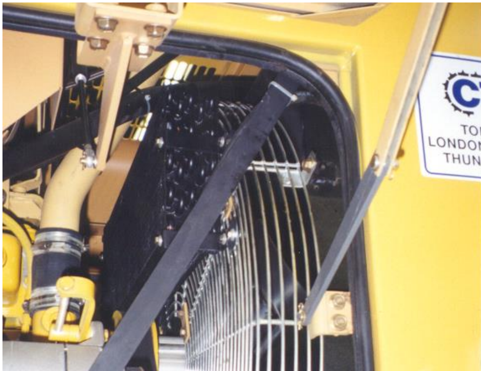
Condenser as viewed from left side.
